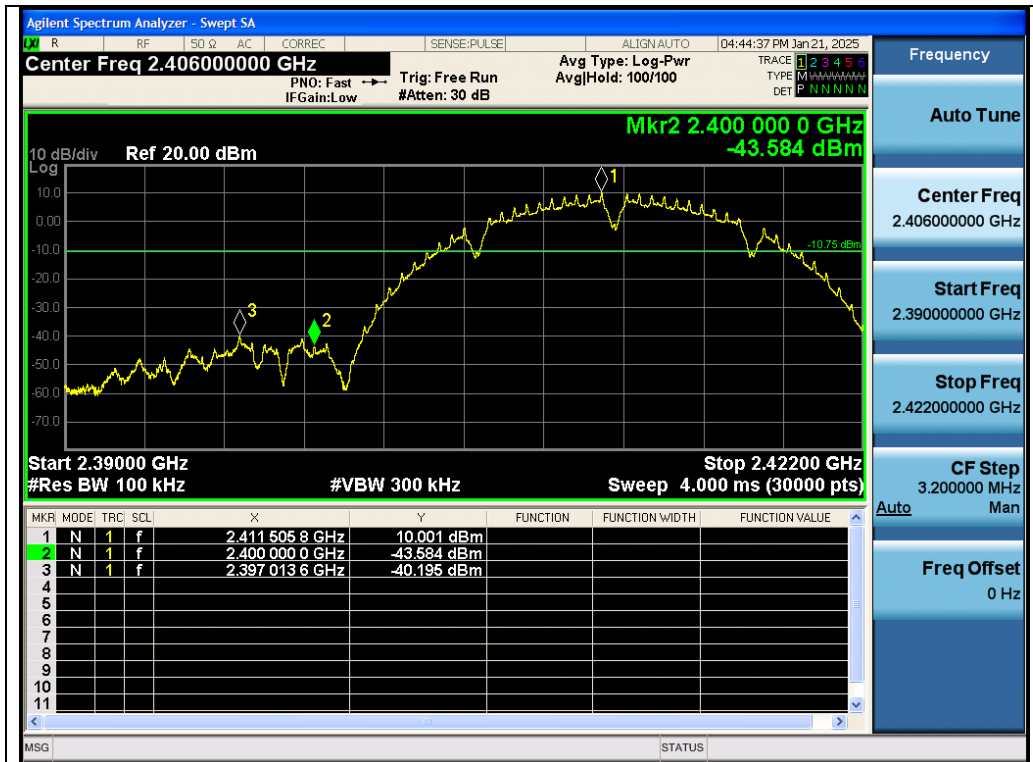
Test_Graph_802.11b_Chain A_2412_1Mbps_Lower Band Edge Emissions
