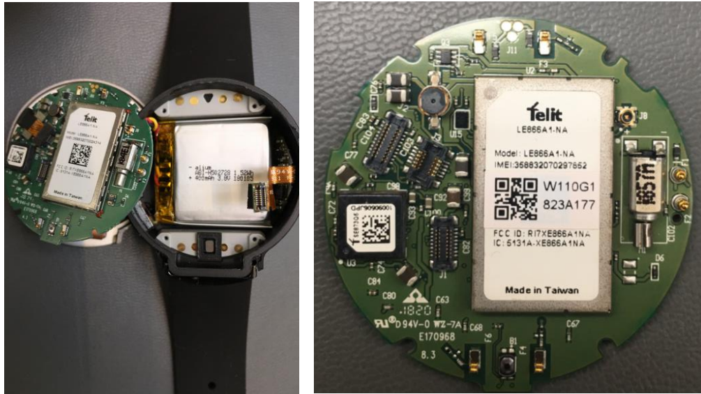
Figure 3 MainBoard backside showing LTE Module (Closeup: LTE MODULE with its FCC ID)
