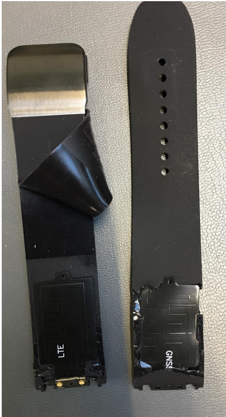
Figure 5 Antenna fabricated on FPC and located in the Straps.
