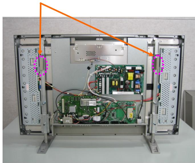
**2. Apply a ferrite Core to the data cable**
