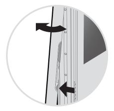
2. Press and hold the rotate button while moving the arm toward the wall
