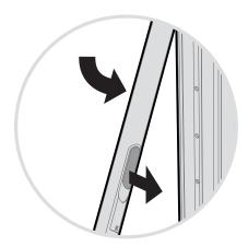
3. Lift angle lever and continue to hold lever to lower arm all the way down
