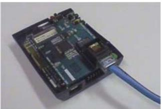
Ethernet cable attached to BlueMod™ internal Ethernet Accessory Card
