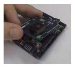
Aligning the BlueMod™ Accessory Board
