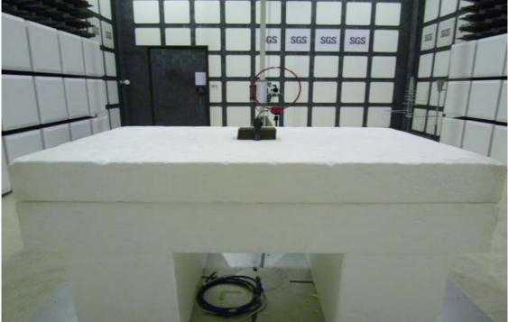
Radiated Emission Set up Photos (Below 1GHz)
