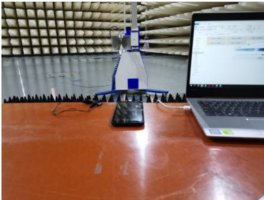
Radiated Emissions Test Setup (above 1GHz)
