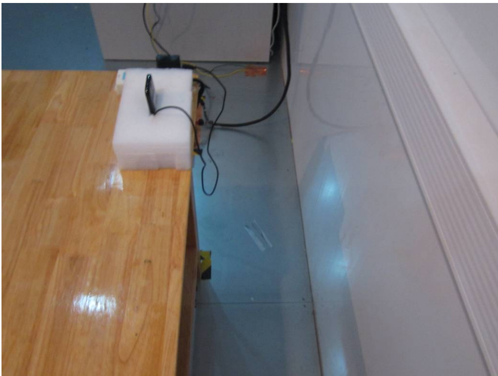
Conducted Emissions Test Setup Side View
