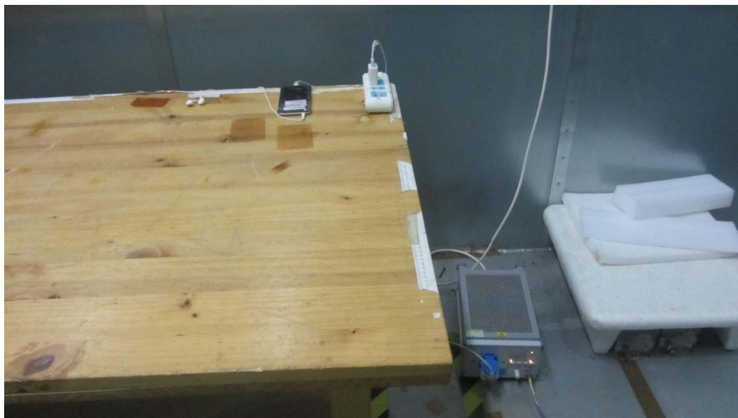
Picture 3 Conducted Emission Test Setup
