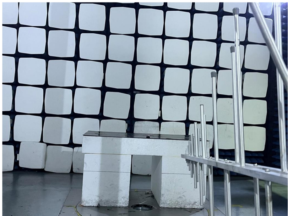
Radiation Emission Test Setup (30MHz to 1GHz)
