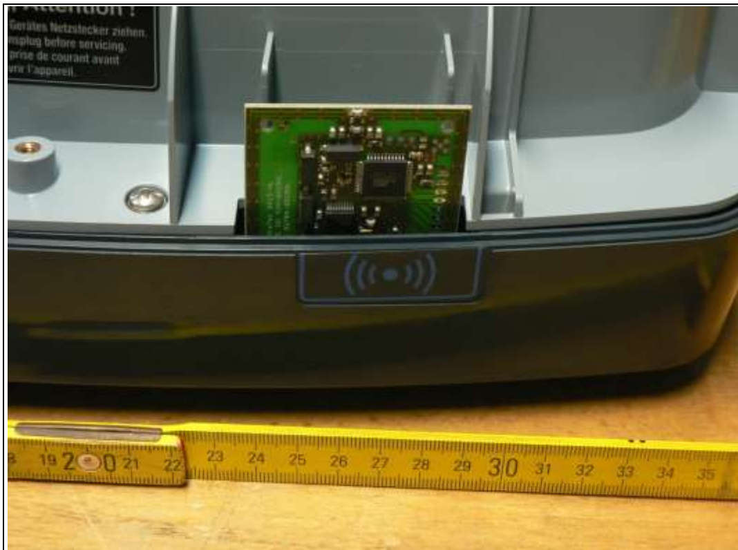
Photograph 3: Placement of RFID Module
