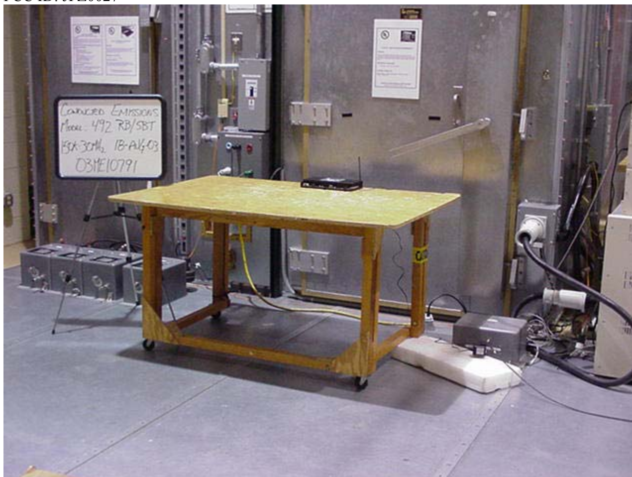
Conducted Emission Test Set-up 150KHz to 30MHz
