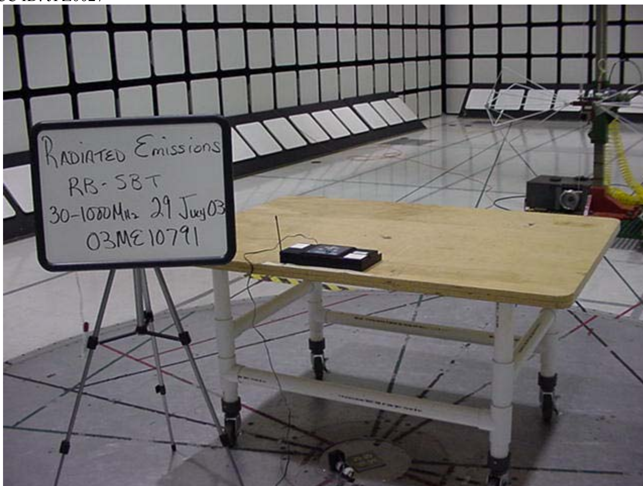
Radiated Emissions Test Set-Up 30-1000MHz Rear View
