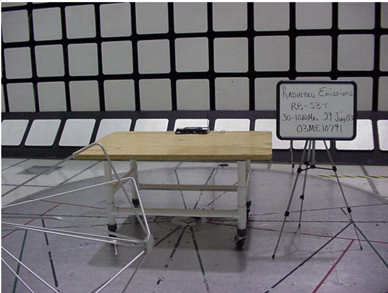
Radiated Emissions Test Set-Up 30-1000MHz Front View
