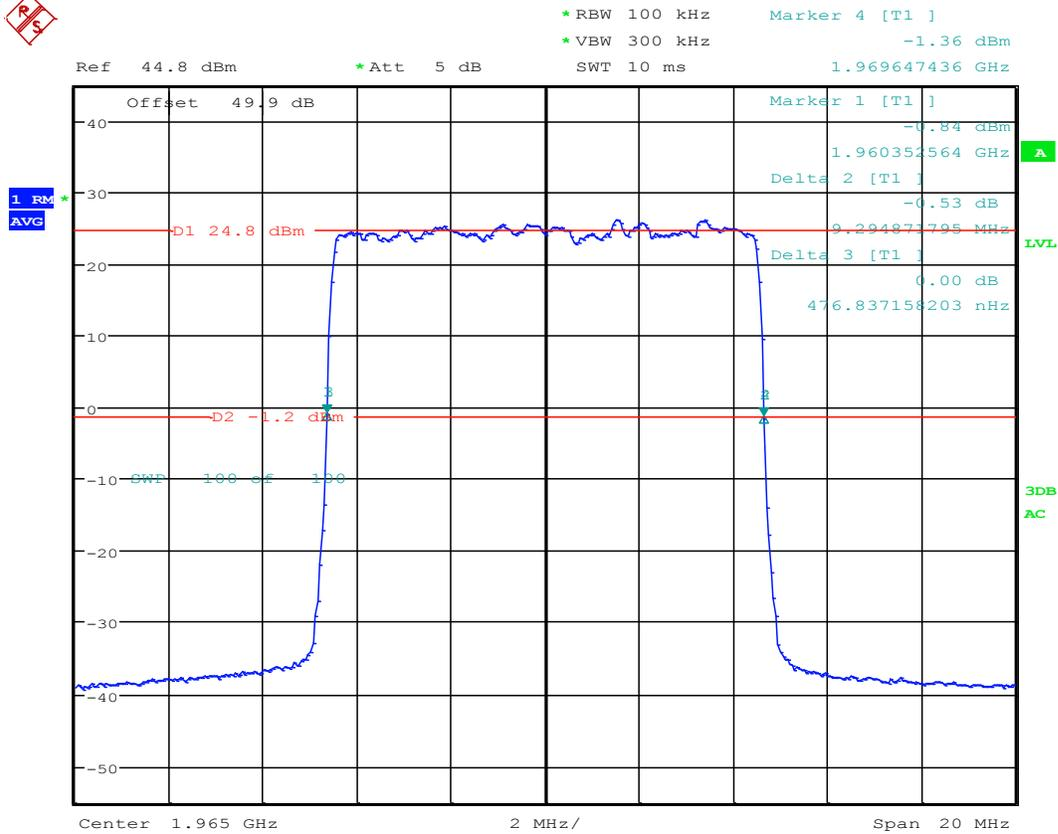
26dB Bandwidth; Test Eng:JY; LTE B25 RRH AR1.0; 1965M
