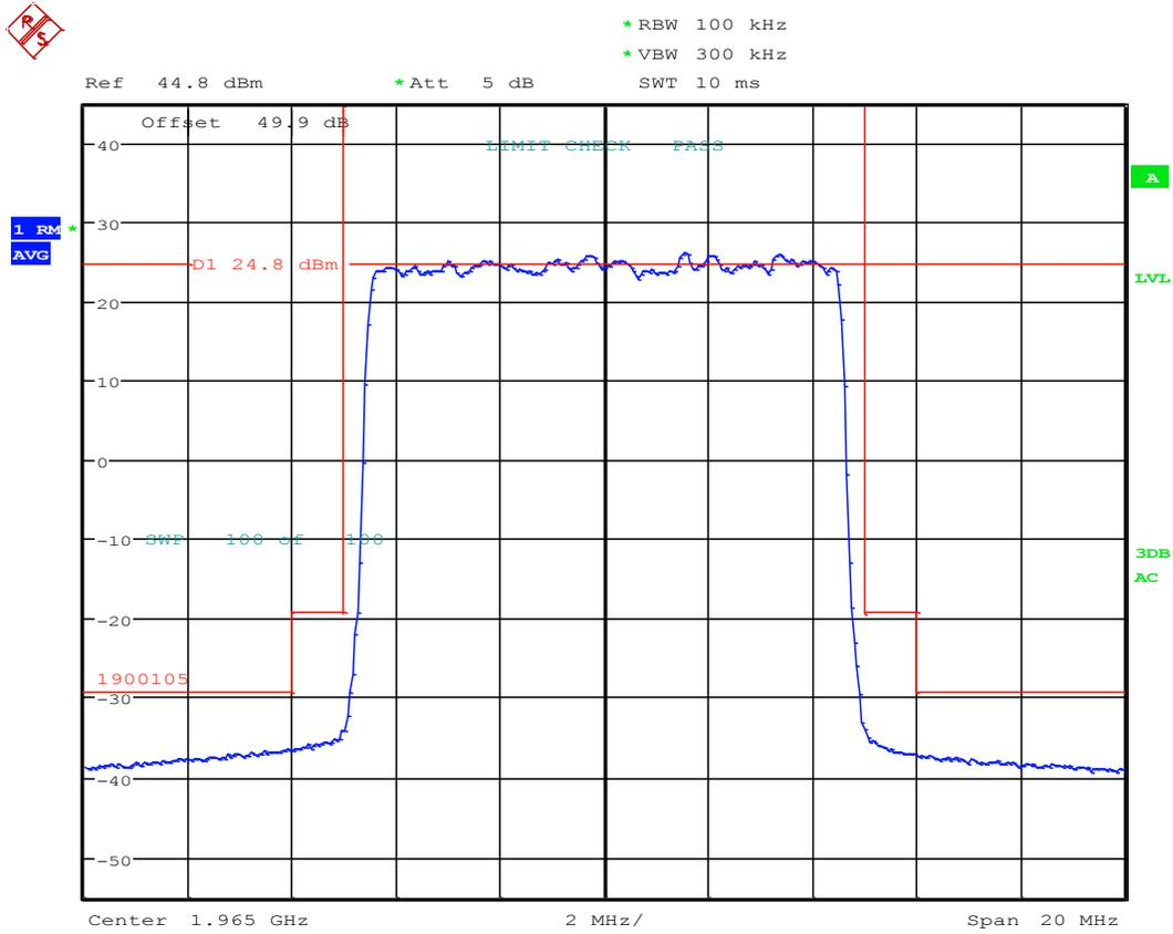
Occupied Bandwidth; Test Eng:JY; LTE B25 RRH AR1.0; 1965M
