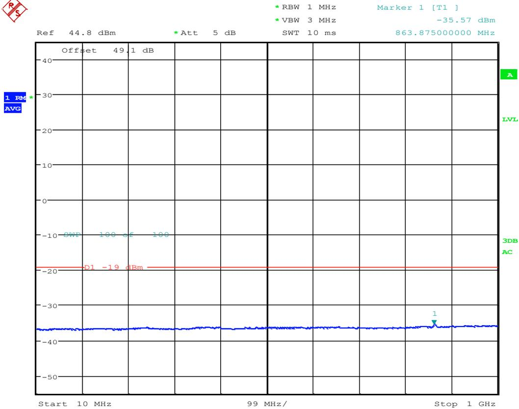
TX Spurious; Test Eng:JY; LTE B25 RRH AR1.0; 1935M
