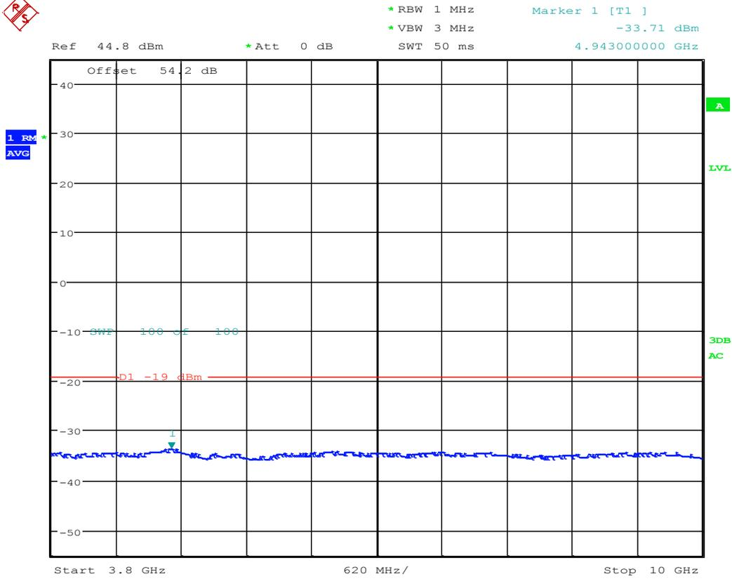
TX Spurious; Test Eng:SG; LTE B25 RRH AR1.0; 1982.5M:64QAM
