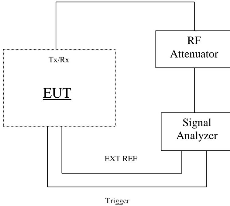
FIGURE 4.2.2 Modulation Measurements
