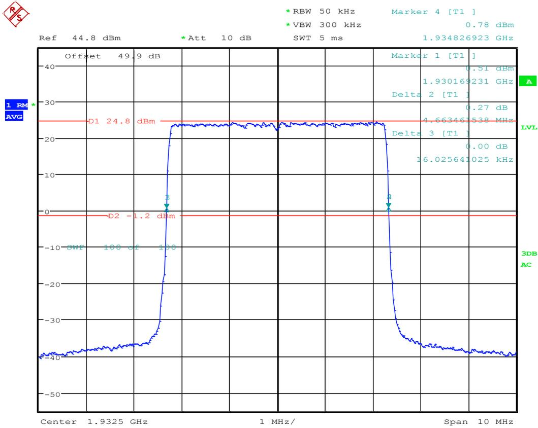
26dB Bandwidth; Test Eng:JY; LTE B25 RRH AR1.0; 1932.5M
