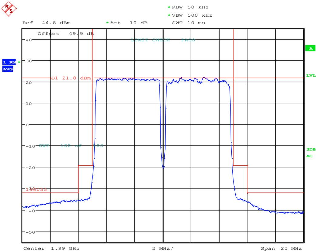
Occupied Bandwidth; Test Eng:SG; LTE B25 RRH AR1.0; 1987.5M:
