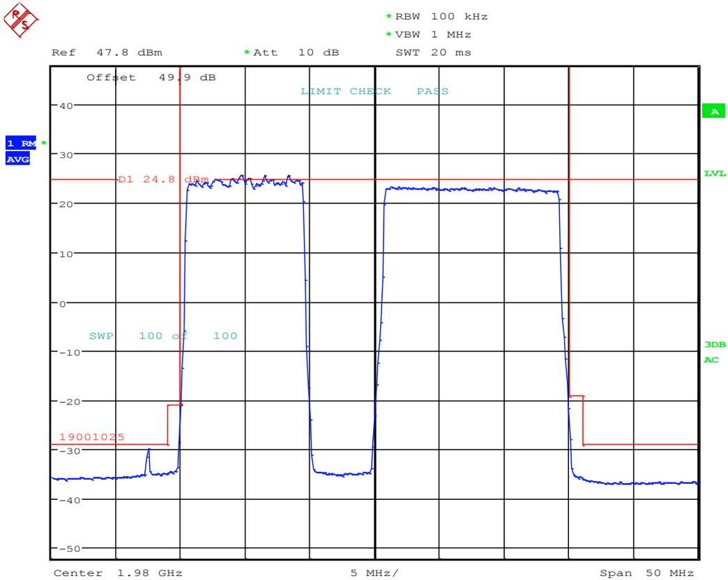
Occupied Bandwidth; Test Eng:SG; LTE B25 RRH AR1.0; 1987.5M:
