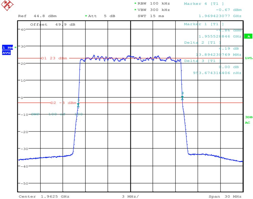
26dB Bandwidth; Test Eng:JY; LTE B25 RRH AR1.0; 1962.5M
