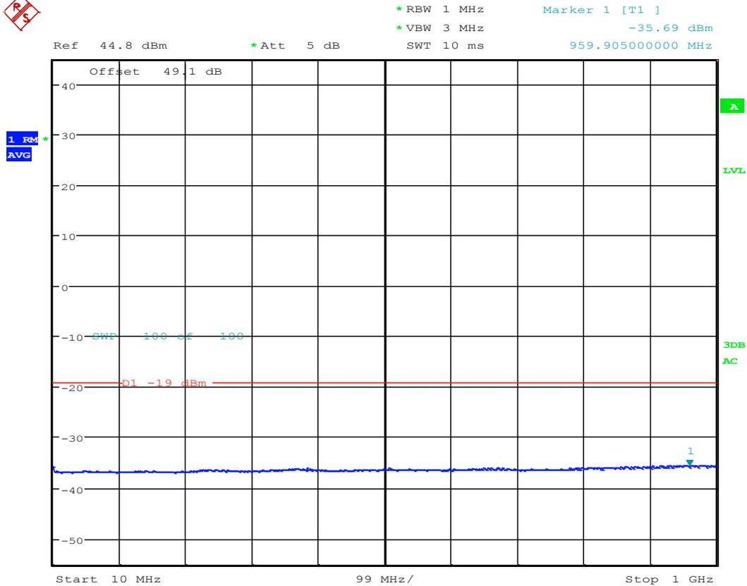
TX Spurious; Test Eng:JY; LTE B25 RRH AR1.0; 1987.5M
