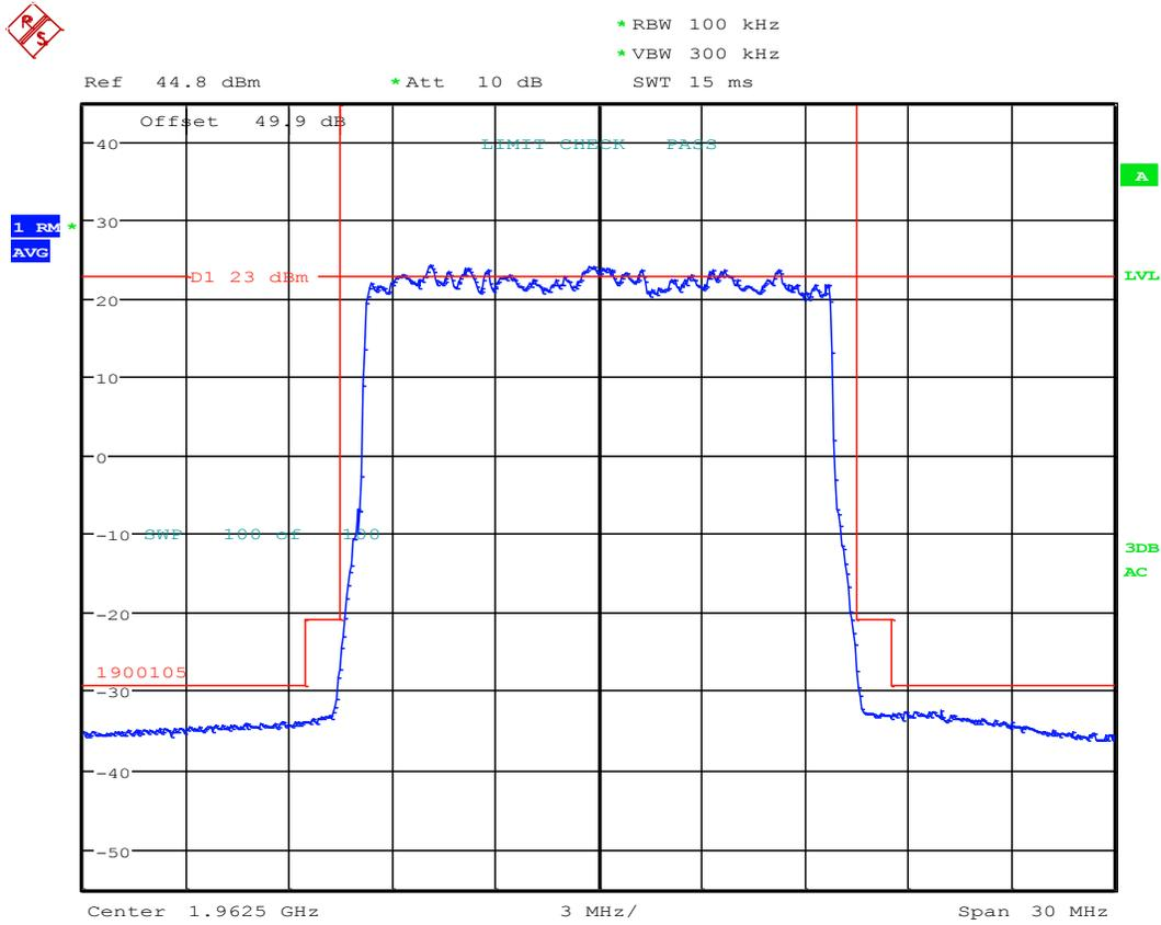
Occupied Bandwidth; Test Eng:JY; LTE B25 RRH AR1.0; 1962.5M
