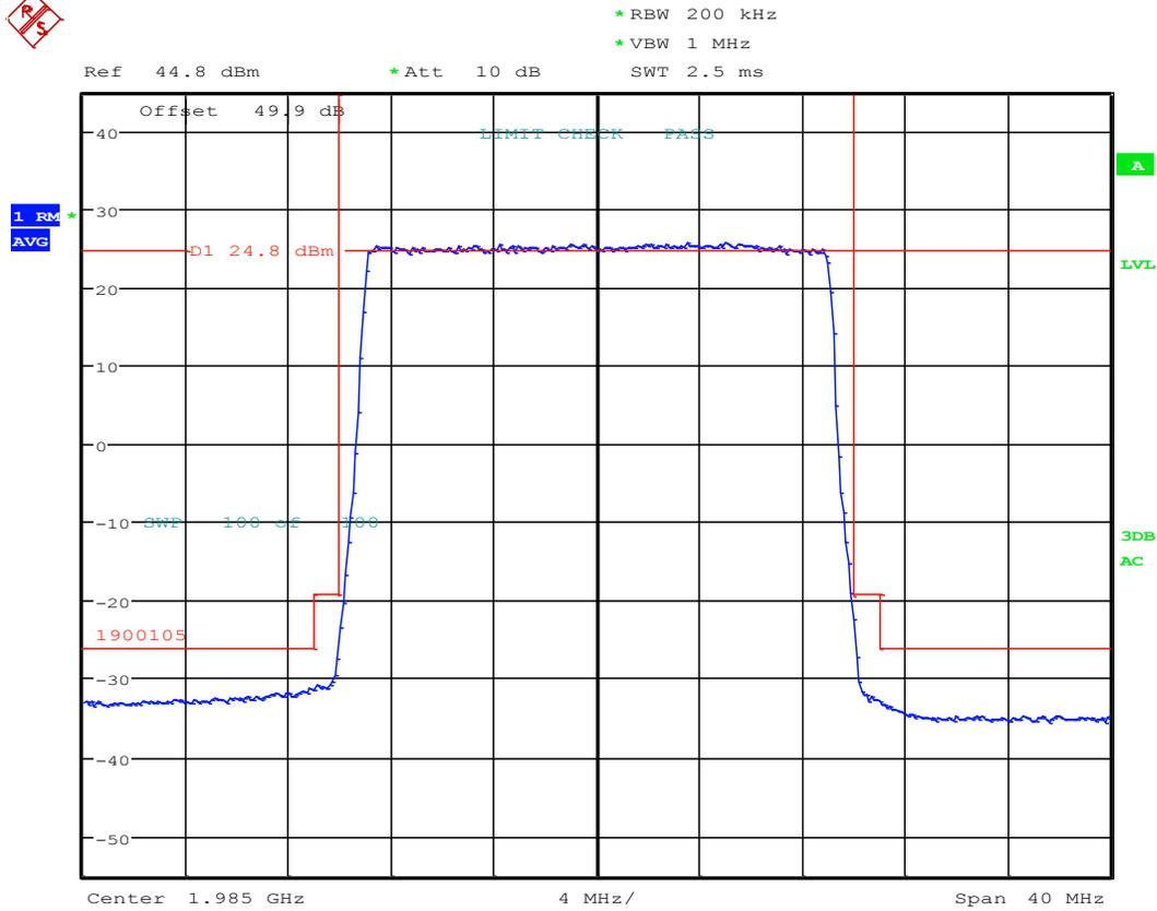
Occupied Bandwidth; Test Eng:JY; LTE B25 RRH AR1.0; 1985M
