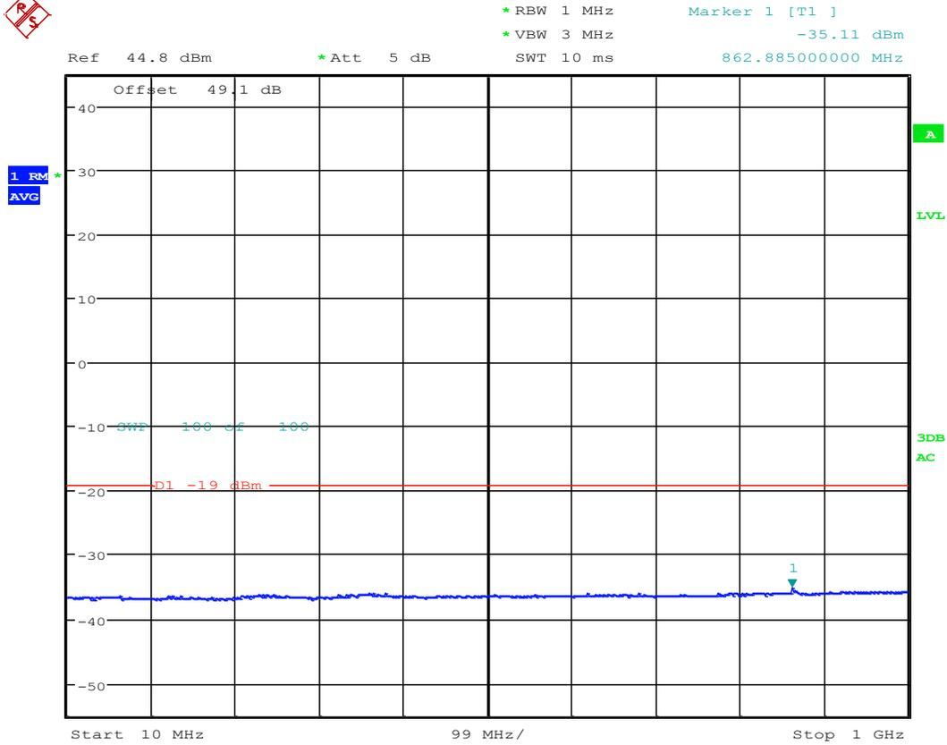
TX Spurious; Test Eng:JY; LTE B25 RRH AR1.0; 1992.5M
