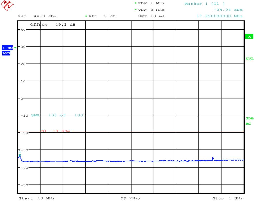
TX Spurious; Test Eng:SG; LTE B25 RRH AR1.0; 1975:64QAM
