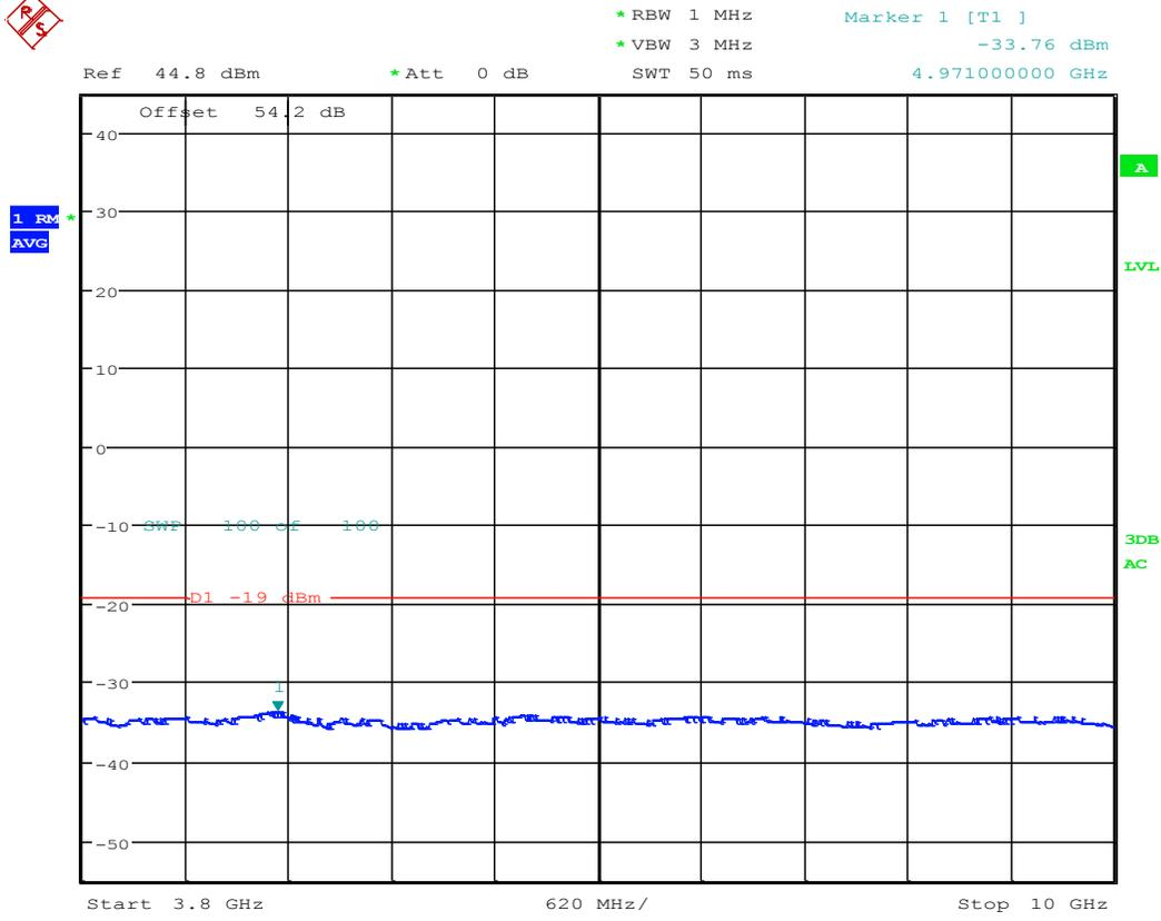
TX Spurious; Test Eng:SG; LTE B25 RRH AR1.0; 1975M:64QAM
