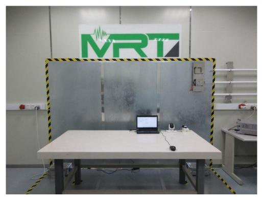
Description: Back View of AC Conducted Emission Test Setup
