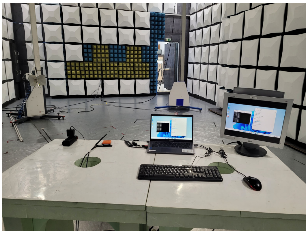
Photo 2: Test setup for radiated measurements below 1 GHz
