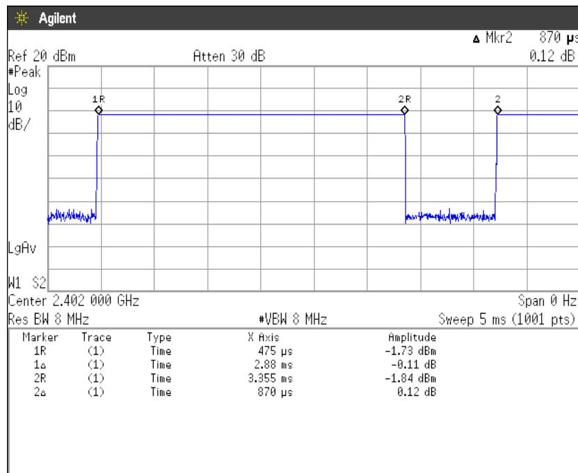
$$\text{Duty Cycle} = \text{Ton} / (\text{Ton} + \text{Toff}) = 2880[\mu\text{s}] / (2880[\mu\text{s}] + 870[\mu\text{s}]) = 76.80[\%]$$
