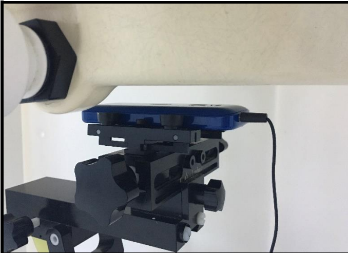
Rear Face of EUT with 1.5 cm Gap_Handset
