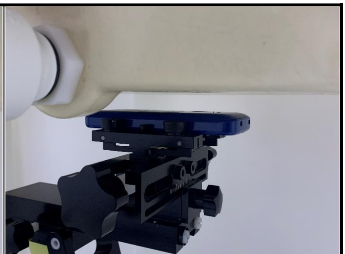
Rear Face of EUT with 1.5 cm Gap
