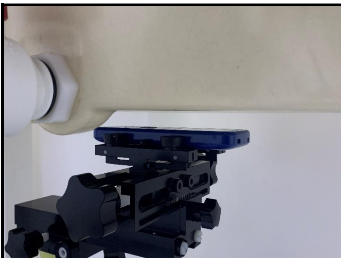
Front Face of EUT with 1.5 cm Gap
