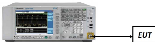
Figure 7-3. Test Instrument & Measurement Setup
