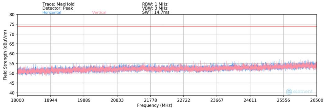
Plot 7-80. Radiated Spurious Plot above 18GHz SISO ANT1
