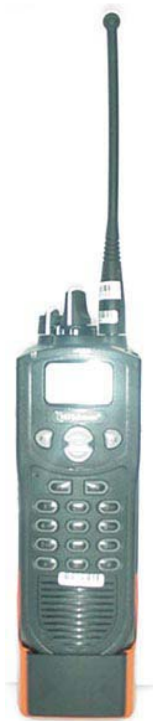
Front of Radio with Whip Antenna & Alkaline Battery Pack
