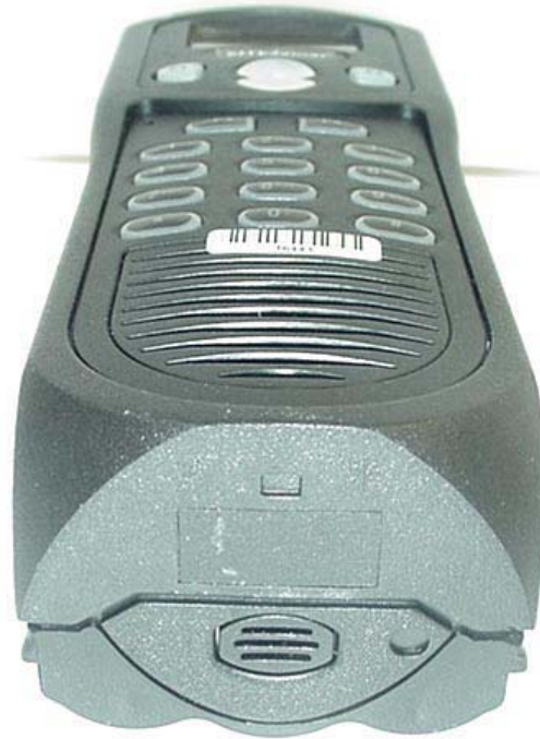
Bottom of DUT with NiMH Battery Pack
