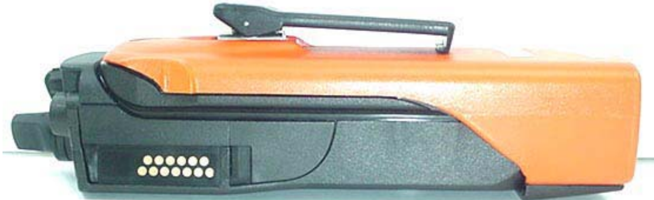
Right Side of DUT with Alkaline Battery Pack & Belt-Clip
