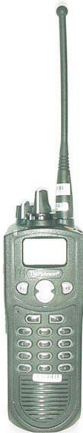
Front of DUT with Whip Antenna & NiMH Battery Pack
