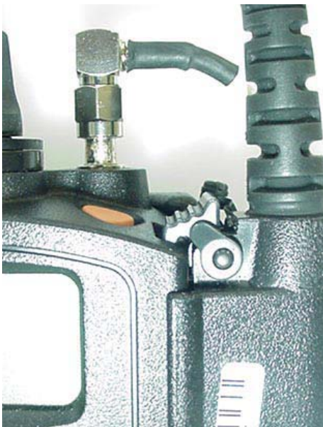
Front View of Antenna Termination
