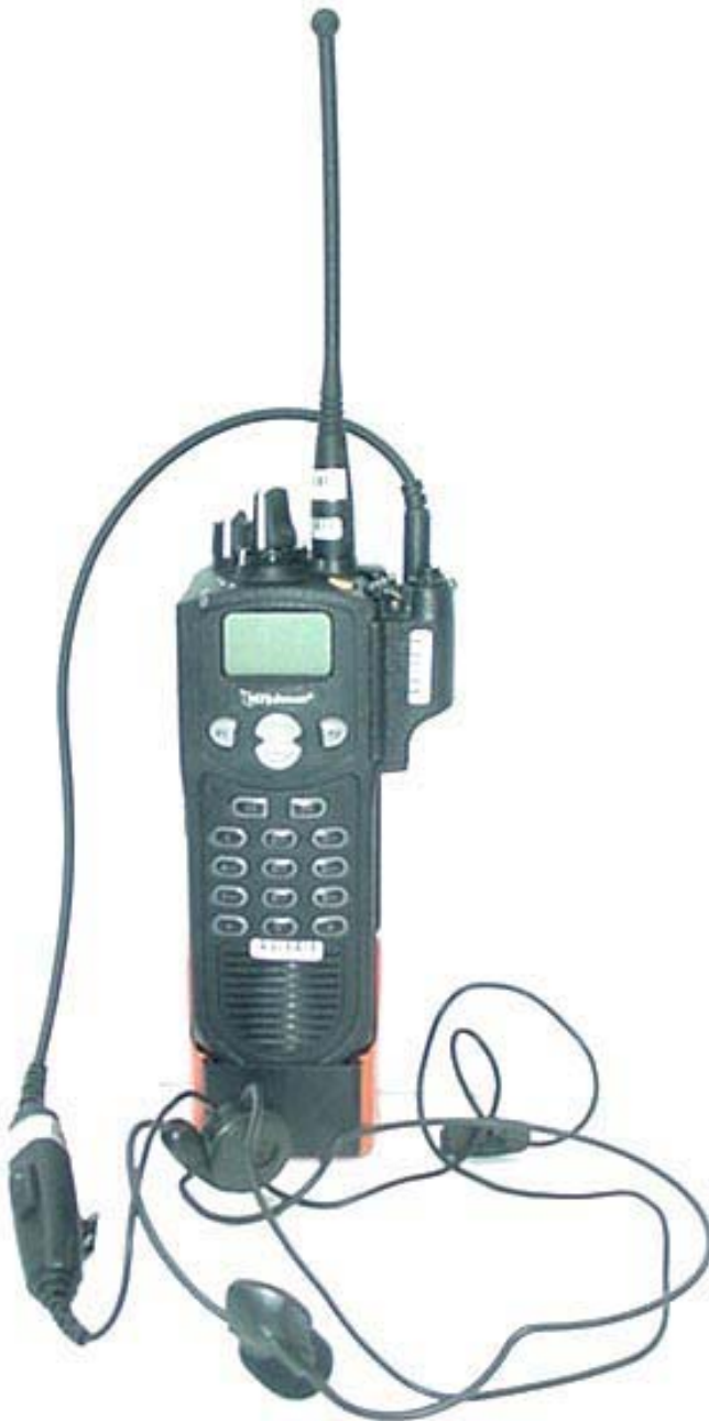
Radio with Boom-Microphone Headset Accessory & Alkaline Battery Pack
