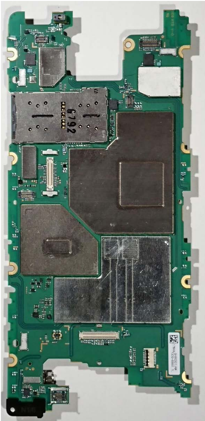
Internal PWB with Shield cases (Front-side)
