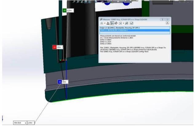
The nominal distance from the bottom of the 900MHz and Wi-Fi antenna to the back plate is 25.95mm:
