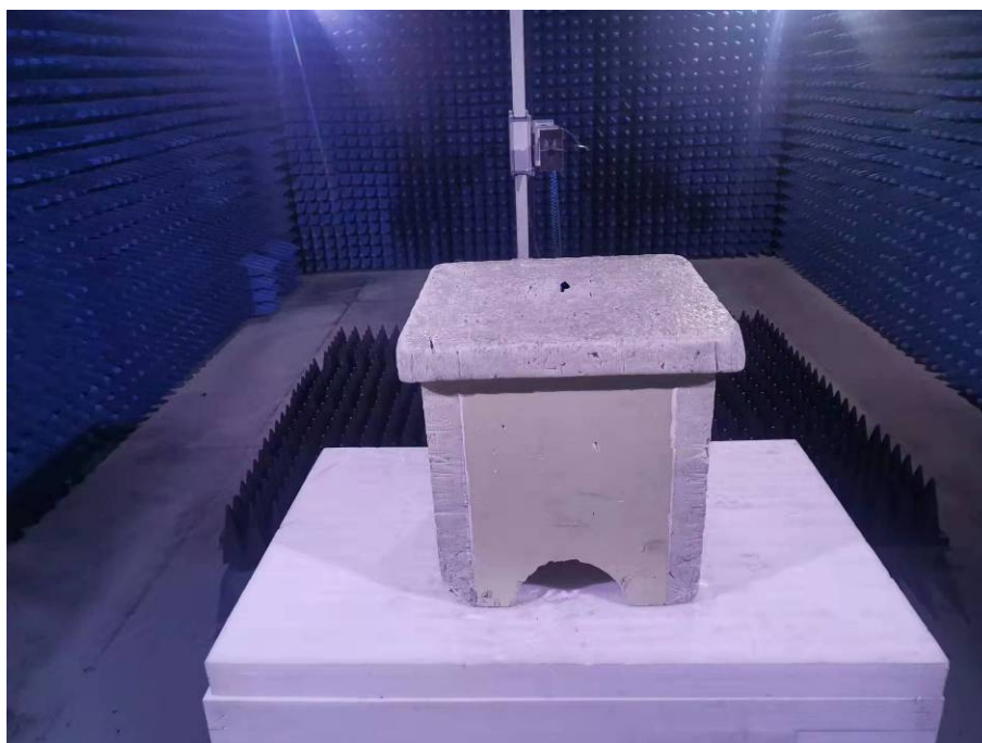
Photo of Radiated Emission Measurement (Above 1G)
