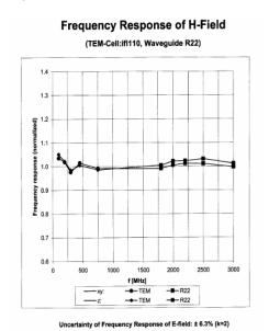
Figure 9 H-Field Probe Frequency Response
