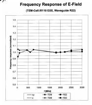
Figure 8 E-Field Probe Frequency Response
