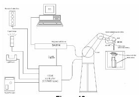
Figure 12 SPEAG Robotic System Diagram
