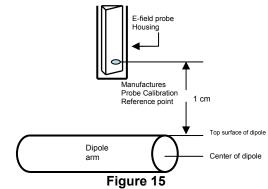
Separation Distance from Dipole to Field Probe
