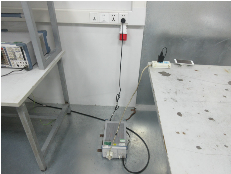
Photo of Conducted Emission Measurement
