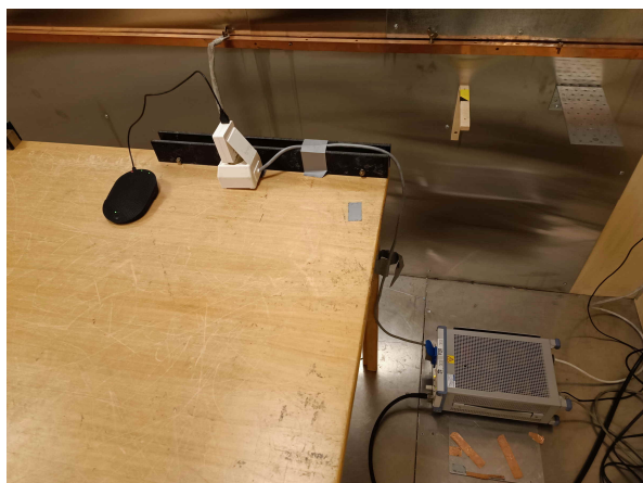
Power-Line Conducted Emissions, WX-ST700P
