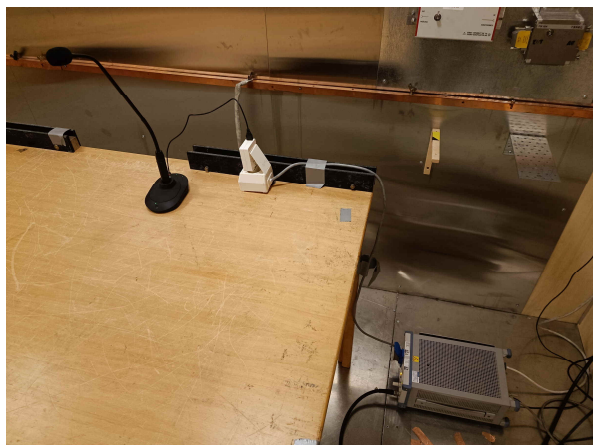
Power-Line Conducted Emissions, WX-ST600P
