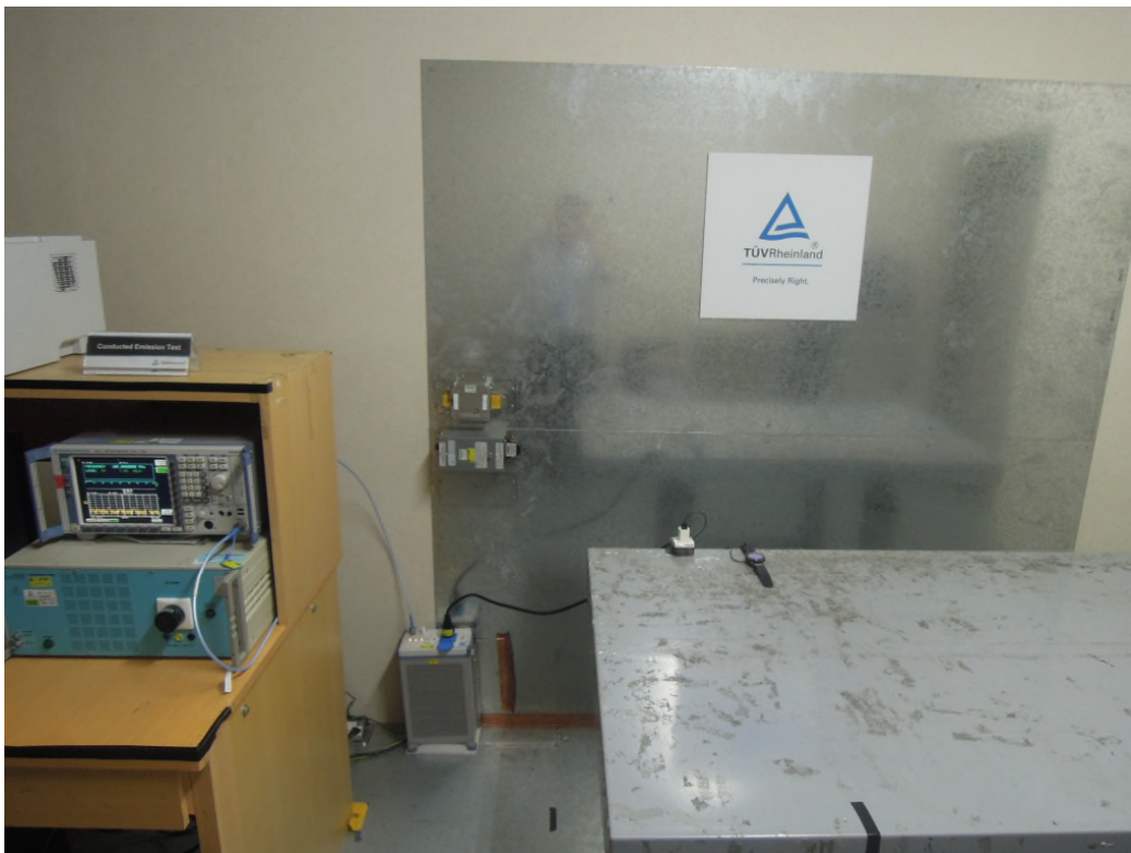
Photograph 6: Set-up for for Mains Conducted testing Front
