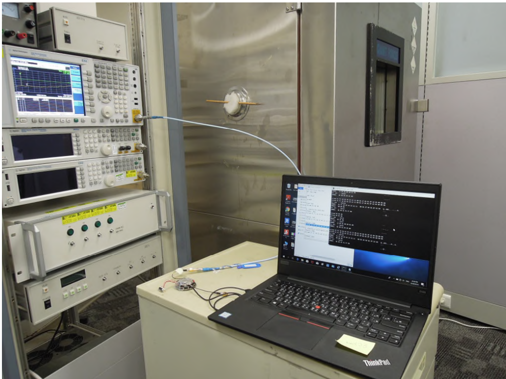
Photograph 4: Set-up for Conducted testing
