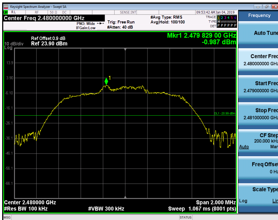
RF Conducted Spurious Emissions_2DH5_2480
