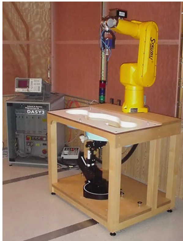
Fig. 5. DASY3 SAR Measurement System
