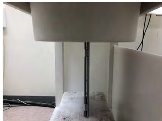
Fig.6 EUT Right side to flat phantom
