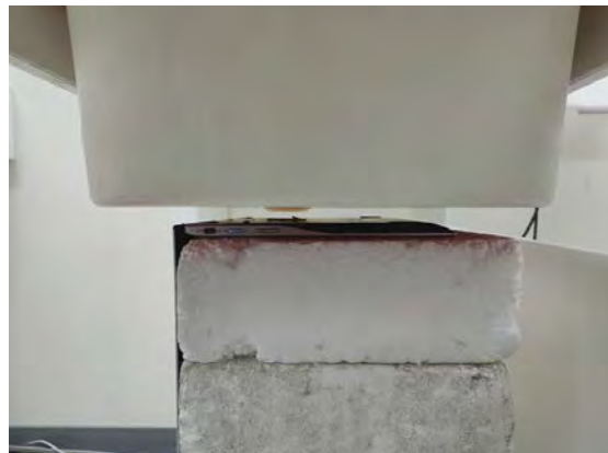
Fig.10 EUT Bottom side to flat phantom
