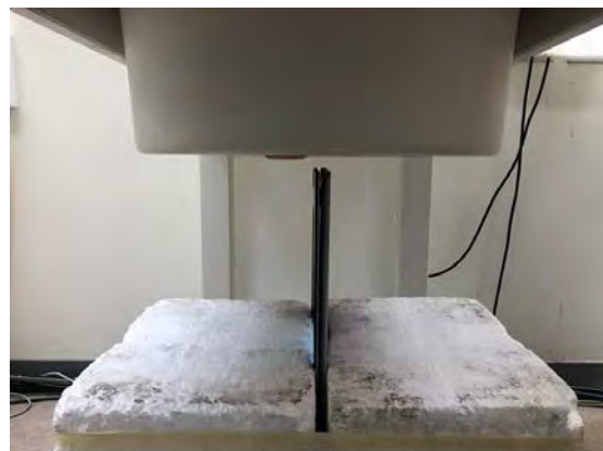
Fig.11 EUT Left side to flat phantom
