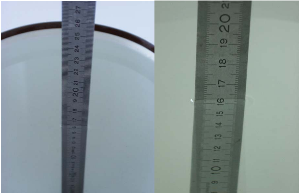
Fig. 62: Liquid depth for PCS 1900 Head and Body measurements.
