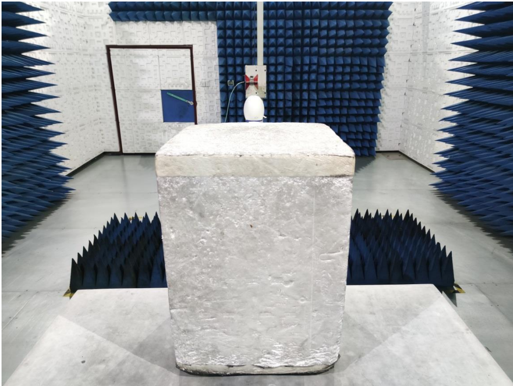
FCC RADIATED EMISSION TEST SETUP ABOVE 1GHZ
