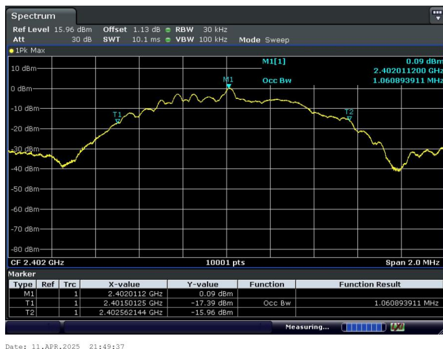
Figure 5. Conducted Emissions, 99% OBW: Low Channel, 2402 MHz Plot
