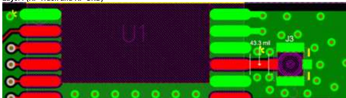
Figure 14: Lyra 24P for External antenna connection host PCB 50-Ohm RF trace schematic with MHF4 RF connector
