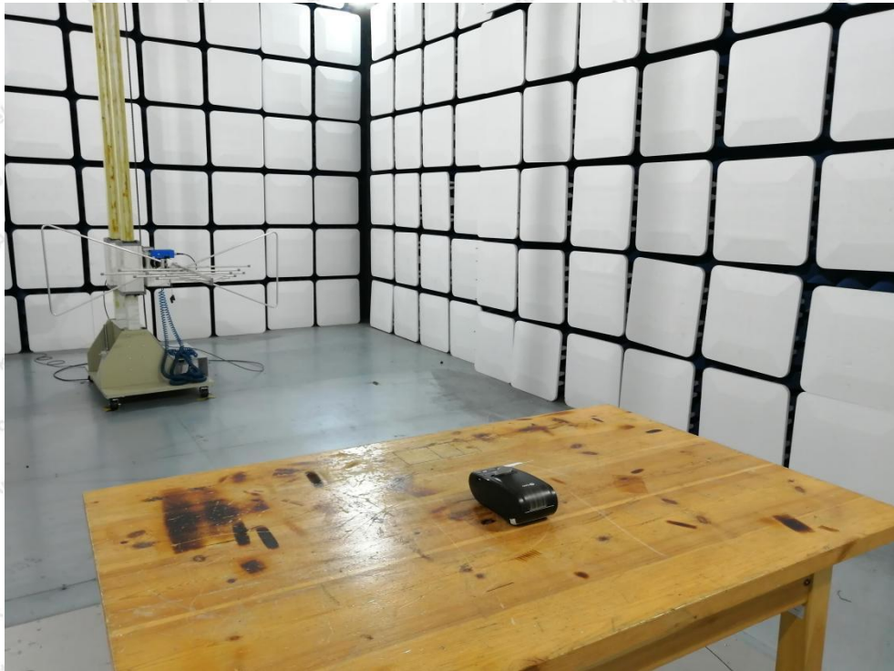
Photo of Radiation Emission Test
