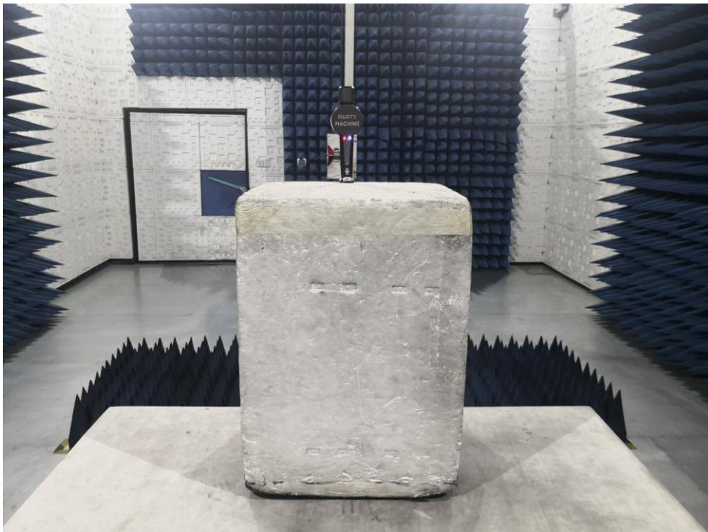
RADIATED EMISSION TEST SETUP ABOVE 1GHz
