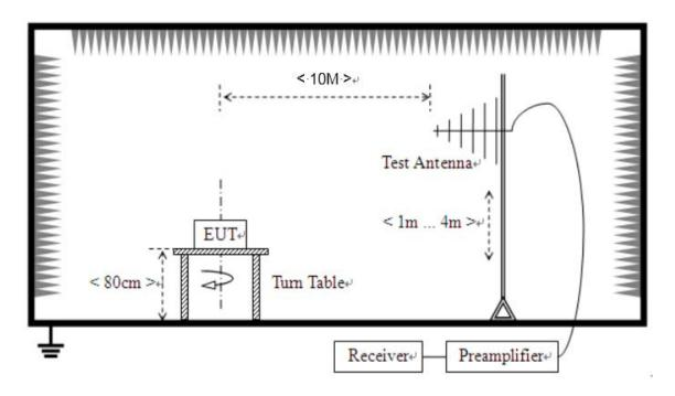
(For Radiated Emission Test (30 MHz-1 GHz))
