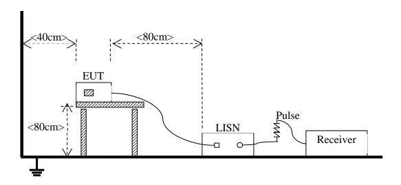
(For Conducted Emission, AC Ports Test)
