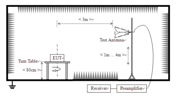
(For Radiated Emission Test (above 1 GHz))
