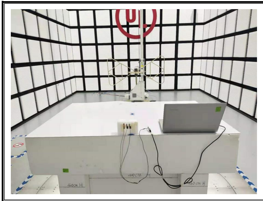
RADIATED RF MEASUREMENT SETUP (Below 30MHz)
