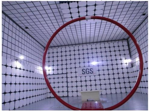
1.3 Radiated Emissions(30MHz-1GHz) Test Setup
