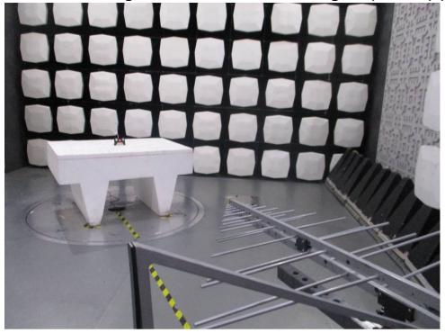
1.2 Radiated Emissions(9kHz-30MHz) Test Setup
