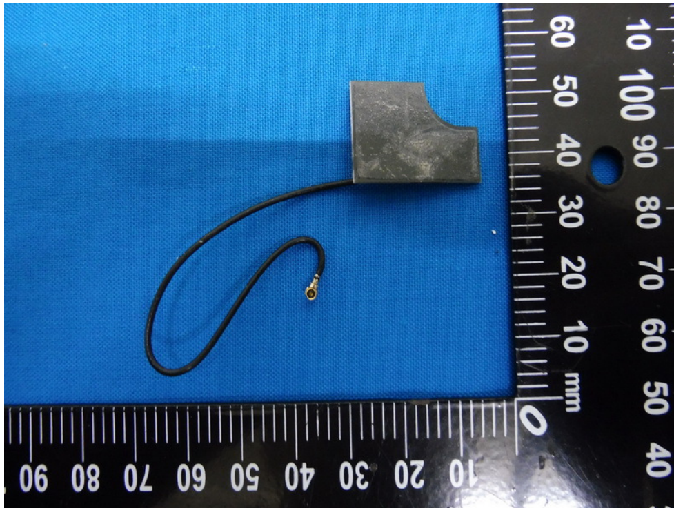
EUT BT& WiFi AUX Antenna location View
