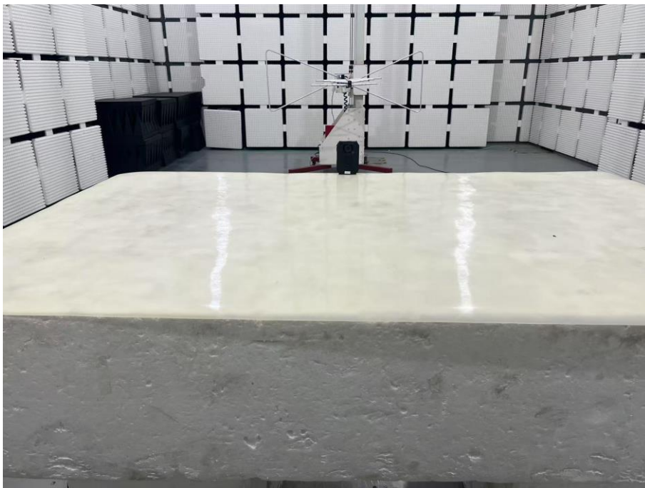
Set-up for Radiated Spurious Emission, Below 1GHz
