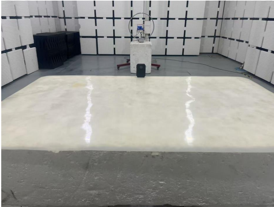
Set-up for Radiated Spurious Emission, Below 1GHz
