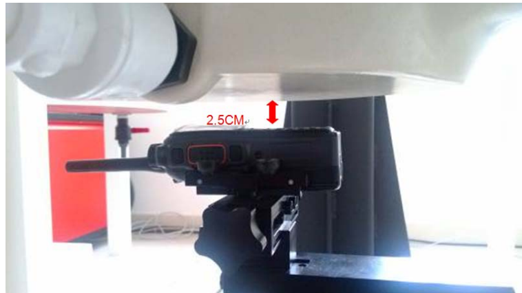
Face-held, The EUT display towards phantom
