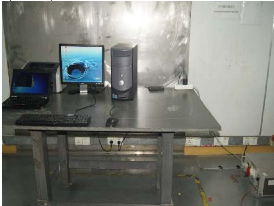
Photograph 2: Set-up for Radiated Emissions below 1GHz
