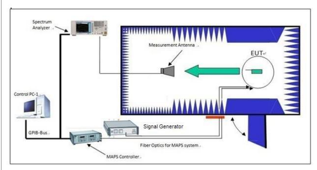
Figure 1. 2D antenna pattern test system.
