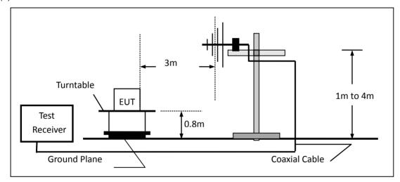
(c) For radiated emissions above 1000MHz
