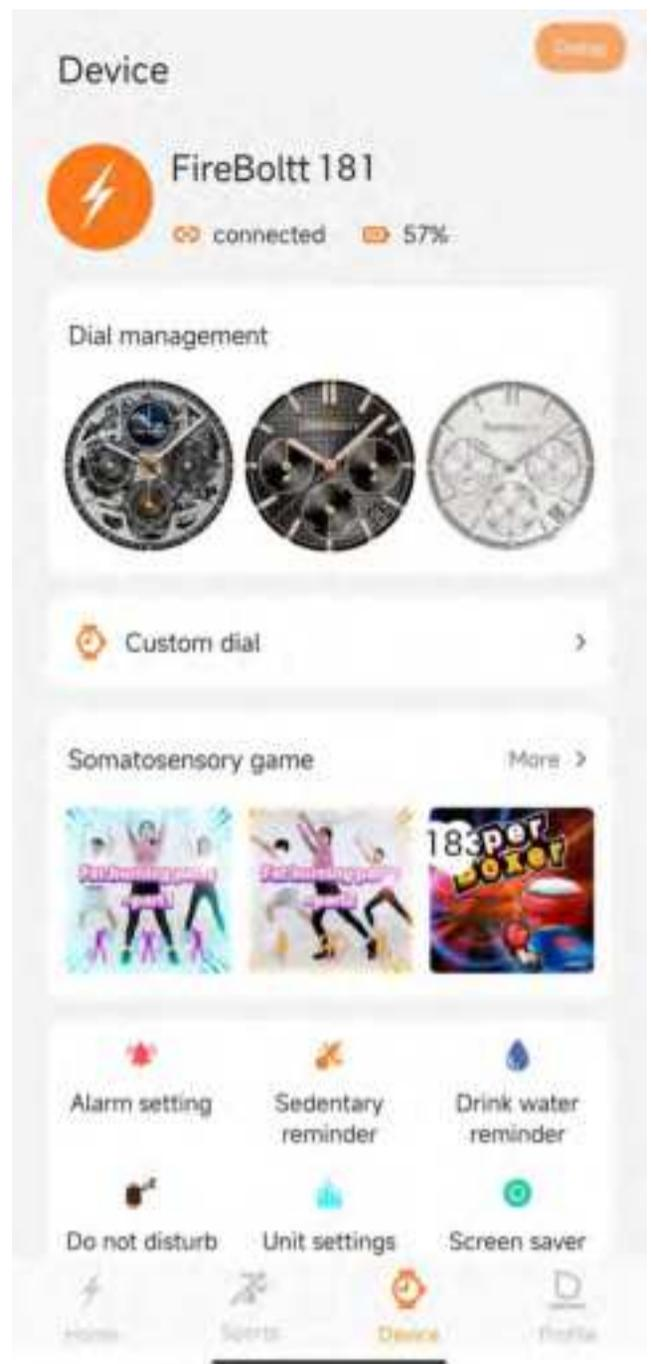
Click the device with correct Name and MAC address (You can check device name from watch setting menu- "About ").After connecting, APP will show device name. And display "synchronizing".
