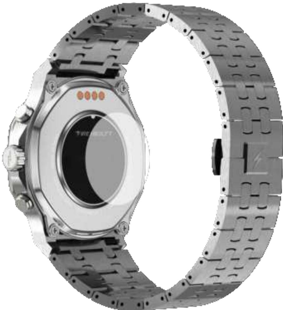
There is a heart rate sensor protector on the sensor, you can take it off before using smartwatch.
