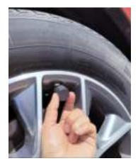
The sensor periodically reads pressure and temperature information. And the sensor periodically sends data via 433.92MHz RF signal.
