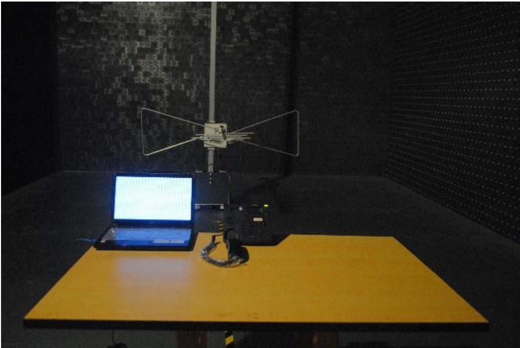
Radiated emission test view (30MHz~1GHz)
