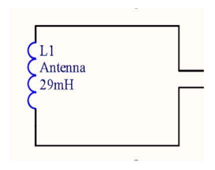
The NFC radio utilizes a loop antenna with an area of about 0.011m<sup>2</sup>. Since the antenna is only generating a magnetic field and not a RF, the gain definition is NA. The antenna coil has 2 turns. The frequency range is 13.56MHz.
