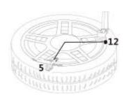
1.7 Apply soapsuds on the valve tip. If no leakage is found, put on the valve cape. If unsuccessful, try again.
