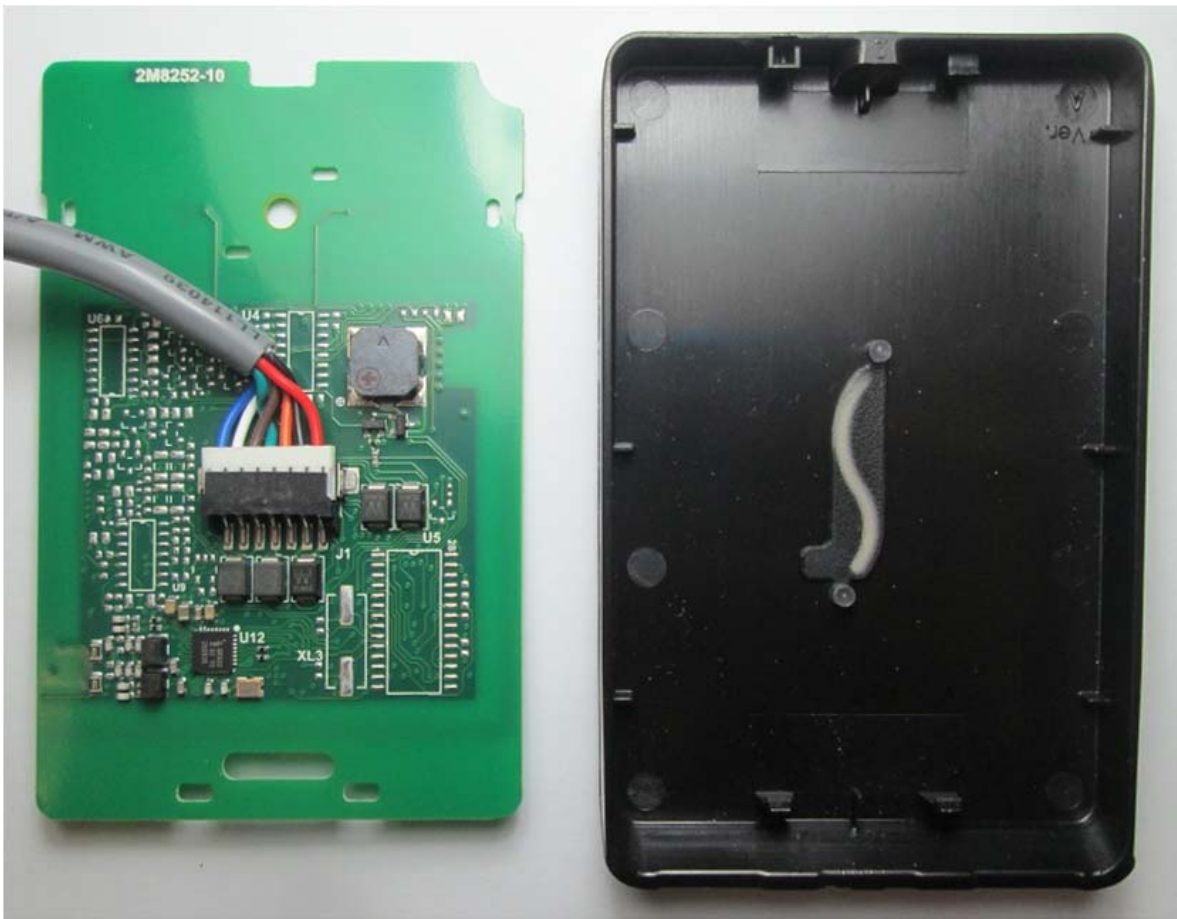
T11 Mifare - Front Cover and PCB Assembly
